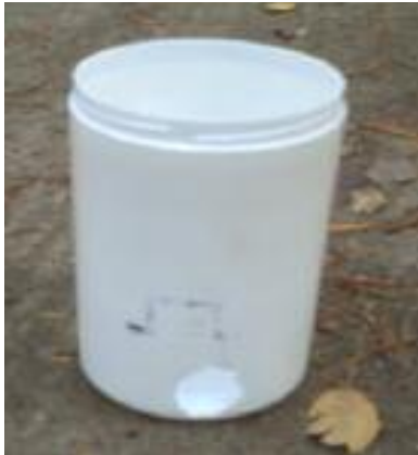
Rocket stand with hole made out of a cylindrical piece of plastic or PBC pipe about 4" long and 3" in diameter.
